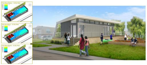
The final Waterlab classroom design achieved 100% daylighting while improving building energy performance Image courtesy of Eskew+Dumez+Ripple
